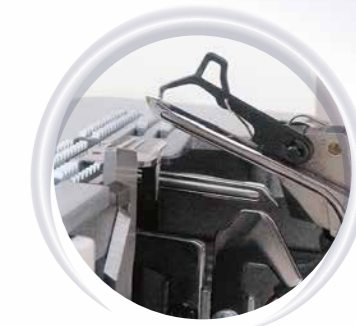
Sturdy looper channels with folding auxiliary looper
