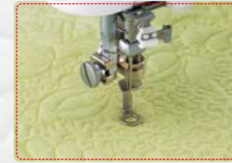
● 1/5" Quilting Foot Use for free motion quilting to glide smoothly and evenly over fabric layers.
