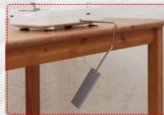
● Knee Lifter Lever The knee lifter lever allows you to lift/lower the presser foot without using your hands. The presser foot can be raised as high as 12mm.
