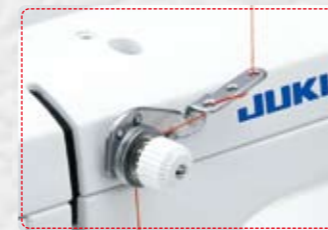
● Sub Tension Unit The Sub Tension Unit ensures thread feeding to the needle is smooth, even and twist free, no matter how thick your thread is. It also keeps the thread from quivering when sewing at high speeds and provides accurate, fine tuned thread tension.
