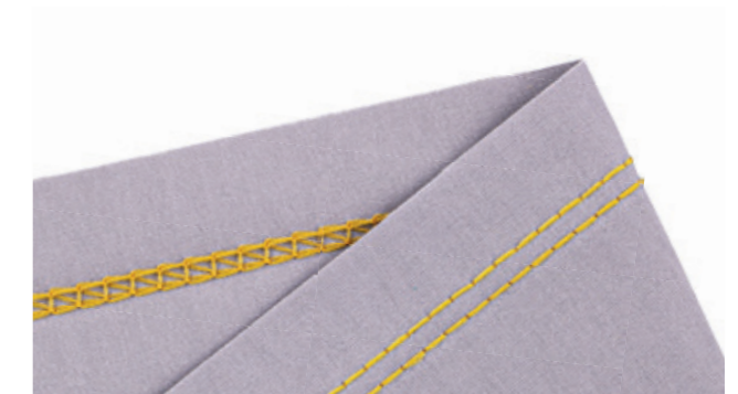
3-thread Cover Stitch narrow (3 mm) for hemming, sewing bindings and decorative effects
