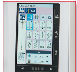
LCD Touch-on kleuren- scherm 110.9 x 62.8mm
